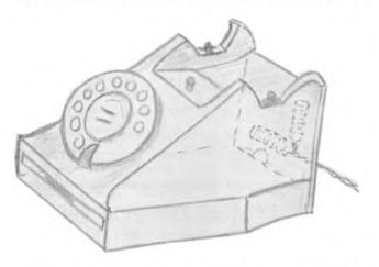
This sketch by Mr. Reid shows two alternative positions for the telephone adaptor. It should be fastened with selotape or elastic.
