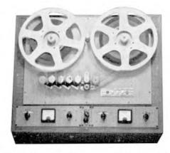
Fig. 8: In this photo the deck is shown, with  $10\frac{1}{2}$  inch N.A.B. spool in position (4,800 ft. of Double play tape!). The two "record" amplifiers are at the foot of the assembly. Left-hand knob in each case is "record" level; right-hand knob is CCIR connection for different tape speeds. The small centre panel holds the main ON/OFF switch and, above it, the erase/record switch for stereo or monaural (top back wipe, or both).
