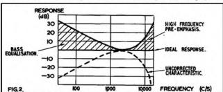
Fig. 2: The fall in response at low and high frequencies (broken line) is offset by bass lift in the playback amplifier, and treble pre-emphasis on recording.
