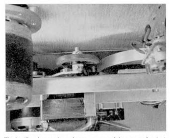
Fig. 9: This close-up shows the arrangement of the capstan fly wheel, the rubber-tyred idler wheel which drives it and, immediately to the left or behind it, the drive wheel of the capstan motor. The general layout can be followed by reference to the other photograph, and by noting that the rewind spooling motor is front left—the forward spooling motor—rear left.
