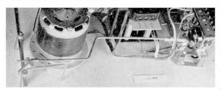
Fig. 2: The brake connection, noted above, can be followed in more detail here, with the tension spring immediately below it. To the left of the spooling motor is the link for that particular brake. Adjustment is effected by slackening off the grub screw and altering the angle of the lever on the shaft.
