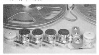
Fig. 7: The layout of tape guides, heads and capstan drive can be seen here, with the tape loop removed. The heads fitted here are (l to r) top track erase; lower track erase; stereo|monaural record; stereo|monaural replay. Between the latter head and the capstan drive is an additional tape guide. Pressure pads and pinch roller are shown in the "stop" or "spooling" position.
