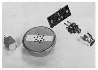
The basic kit of components includes the head, microphone/earpiece, transistor, plug, socket and cover.
