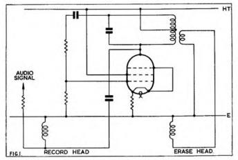
Fig. 1. Circuit of oscillator for low impedance heads.
