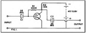
**R2** is the collector load resistance. This is not critical within a few thousand ohms, i.e. anything between 7 K and 15 K will do.
