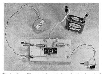
Showing the amplifier set up for use to boost the microphone signal into radio or loudspeaker.
