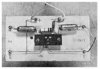
This close-up of the breadboard shows the wiring and will help to identify each component on the circuit diagram.
