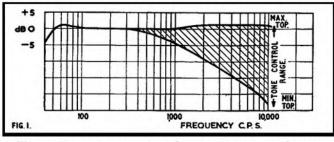
Fig. 1. Frequency response on replay, showing tone control range.
