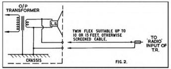
Fig. 2: The correct way to use Ext. L/S terminals.
