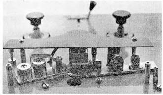
Close up of the sound channel shows the twin permanent magnet erase heads (left), the record/replay head, and pressure roller.
