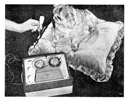
THE subject of this month's field trial is bigger, heavier and costlier than the previous models, but the extra facilities offered make these factors relatively unimportant. After all, the Minivox still weighs less than 10 lbs., and measures only  $10\frac{1}{2} \times 5\frac{1}{4} \times 9$  in. It presents a very smart appearance, in two tones of grey, and the sloping top gives an impression of slimness to the whole machine.
