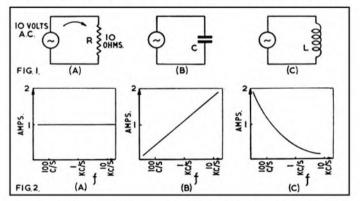
resistor is the number of volts required to drive 1 ampere of current through it. (See figs. 1a and 2a).
