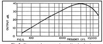
Fig. 5. Uncorrected response of record/replay heads
