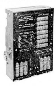
battery may be used, or a mains adaptor is available to run the recorder from 220 or 110 volt AC mains.
