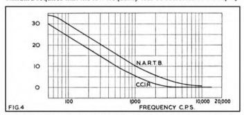
Fig. 4. Replay characteristics for the two standards now in use.
