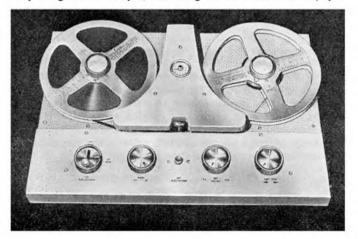
chronous or alternatively hysteresis synchronous, and two side motors. Instant start and stop is possible. The only other moving parts are the pinchwheel and a gear-driven clock-type tape position indicator. The main motor, which is direct drive can be reversible and provision is made in the head assembly unit for 3 heads to be accommodated each side of the capstan.
