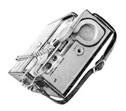
batteries. Six of these supply the amplifier, and have an operating life of approximately 300 hours. The remaining seven batteries operate the motor, and will last for about 50 hours. For fast wind and rewind, the motor voltage is doubled. The winding time was found to be 40 seconds and 90 seconds for rewind and wind-on respectively, with the standard tape supplied.
