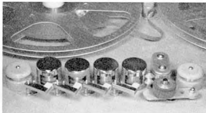
"... bring a pencil up to the capstan while it is running."
