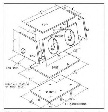
This exploded diagram of the case indicates the pieces required and the basic outline of assembly. Future photographs and diagrams will show the detailed construction.  $\frac{1}{4}$  in. oak was used throughout.
