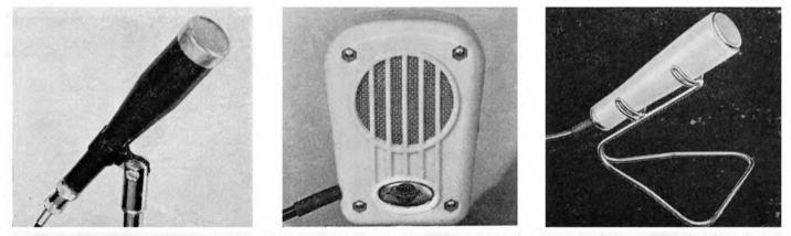
Three popular microphones which illustrate the contrast in styles referred to in the first letter on this page. Reading from left to right they are the Grampian DP4 moving coil, the Lustraphone DL66 moving coil, and the Acos Mic 39-1 crystal.
