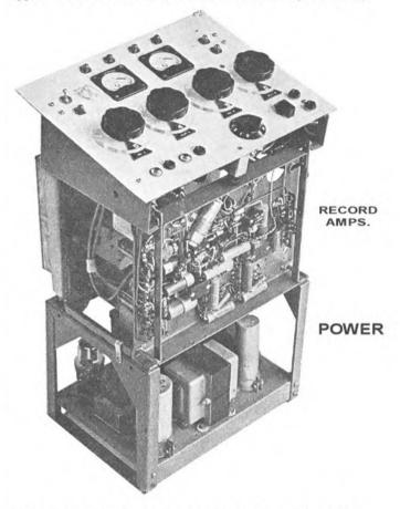
Fig. 2. View of the main chassis showing the record amplifiers.
