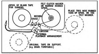
containing the original programme on a holder of some sort (gram turntable?). Lead this tape past the external PB arrangement, on to and past the capstan (or pinch wheel) and finally to a take up spool of greater hub diameter than that being used for the dubbing tape. Place the programme take up spool on top of the dubbing take up spool, separated by a felt washer to act as separator and clutch.
