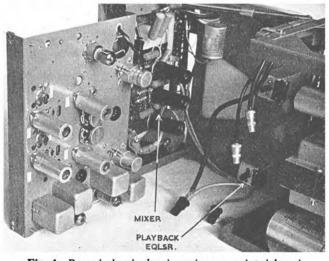
Fig. 4. Record chassis showing mixer on printed board.
