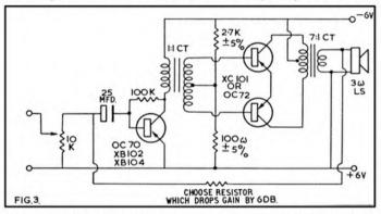
shown in Fig. 3. A little negative feedback is applied to reduce distortion to the lowest possible level at medium power outputs.
