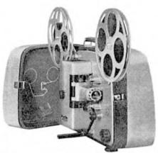
THE Specto-Royal 8 mm projector is very neatly designed with a two-tone laminated case. It is easy to carry and the plastic handle will lie flat on top of the case when not being used. The side-cover is easy to remove by means of the two Cheney clips and contains a 9 ft. mains lead. There are two spool arms with 400 ft. capacity which fold out from the chassis, each with its own rubber driving belt. Weight—12 lbs.
