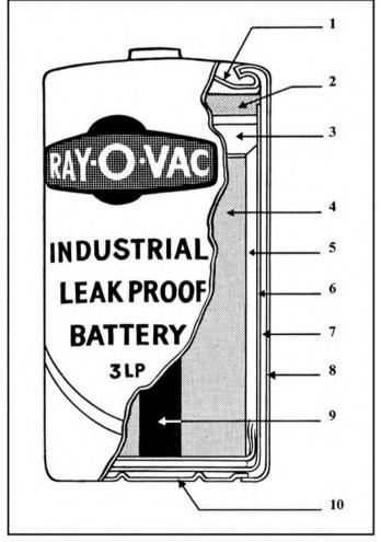
Steel top cap. 2. Plastic seal. 3. Air space. 4. Manganese dioxide.
