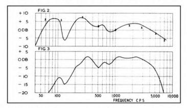
a signal 12dB above test tape level could be recorded with negligible distortion. This means that tapes recorded on this machine show a signal/noise ratio of better than 40dB on wide range playback equipment, and 36 to 37dB when played on the portable recorder.
