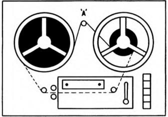
Position A shows new tape guide for modification to Truvox.
