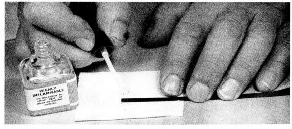
IN the previous article I dealt with editing and the splicing of tape using a pressure adhesive jointing tape. It was explained that this type of joint is of a temporary nature, since it can if necessary be taken apart and then remade without damage to the recorded material. However, there is another method type which can be used—the permanent joint—so called since once it has been made there is no way of taking it apart without damaging the tape.
