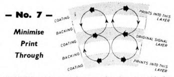
UNLESS certain precautions are taken there is a risk that when a recording is spooled up, the signal on one layer of the tape may print an attenuated copy of itself into adjacent layers. In really bad cases the print signals may penetrate up to five or more layers on either side of the original, giving a disconcerting pre-echo or post-echo effect.
