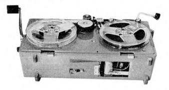
Photo 4: View showing cover removed, battery door open, and wind and re-wind handles extended.
