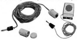
Fig. 3: Extending a microphone lead using a film container, jack socket and screened cable.
