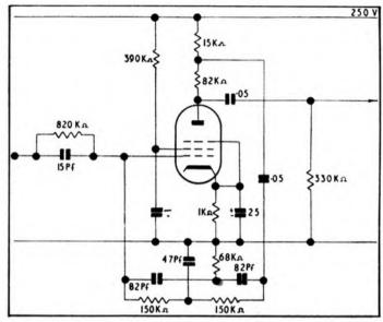
FIG. 2: A single valve, Bridged-Tee circuit.
