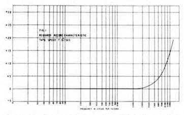
fier, resulting in a curve similar to fig. 1. This is the curve that may vary from one machine to another, depending upon the tape in use, and the particular qualities of the head used.
