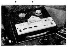
The Sound Riviera is a compact tape recorder operating at 3<sup>1</sup>/<sub>4</sub> i/s and capable of 3 hours recording and play back time. Over 3 watts output is available from the elliptical loudspeaker. Frequency range claimed is from 40 c/s to 10,000 c/s. Facilities include, monitoring from headphones, output for external amplifier, extension speaker sockets: inputs for microphone, radio/ gram, record player and telephone pick-up, edge-wise controls and a Magic Eye.
