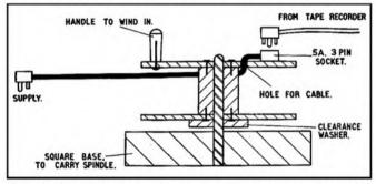
face of the drum, this being wired up to the inner end of the cable, the idea being to disconnect the short tape recorder cable from the extension, thereby leaving the drum free to be wound up by means of the handle provided. The great feature of this arrangement is that the cable is wound up without twisting its core. I hope you find this idea useful. Yours faithfully.
