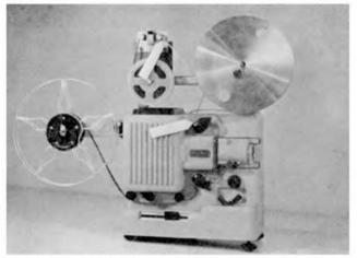
Stage 3. The prepared tape end is anchored in one of the slots of the flywheel with the white leader within one inch of the sound head. The junction of the black leader with the film is on the top sprocket of the projector. See arrows.
