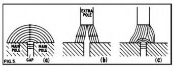
Fig. 5. Flux pattern in a Cross-Field Head. (a) Diffuse field due to main poles. (b) Cross field between main and extra poles. (c) Resultant concentrated field.
