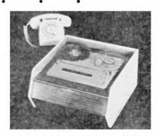
A NEW telephone answering machine—the first British production to employ printed circuits and transistors in its construction—has been announced by Robophone Ltd. of Tottenham Court Road, London.
