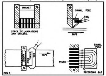
Fig. 3. Recording Head for Boundary-Displacement System. The magnetic circuit through the high-reluctance lamination/spacer stack is shunted by the adjacent signal pole, each half carrying flux in opposite directions with a neutral point in the centre, thus: Energising the signal pole produces a uniform field component which adds to one half of the standing field and subtracts from the other, thus shifting the neutral point from the centre.
