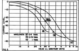
Fig. 2. Transfer characteristics of Carrier-Erase Recording. Carrier level vs head d.c., wavelength as parameter. (0.75 thou' is equivalent to 10 Kc/s at 7½ i/s, for example.)
