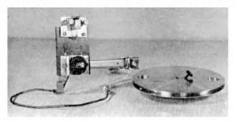
The hardware: The flywheel cum tape spool (right) measures 5½ in. in diameter, weighs 1 lb. and carries a ½ in. by ½ in. slot on its outer rim to hold the tape. The head unit (left) is made up from standard "Portable Recorder" kit items. The magnetic head, head plate with tape guides and pressure pad, together with the supply reel spindle and bracket, are mounted on a platform with a means of clamping to the supply reel arm of the projector.
