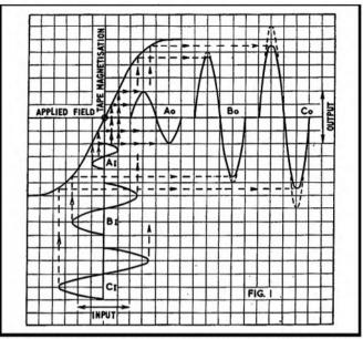
Fig. 1. Heavy curve at top left shows magnetisation curve (transfer characteristic) of A.C. biased tape. Input waveforms A, B, C result in output waveforms A, B, C. Peak distortion suffered by B and C; dashed "caps" show correct waveform peaks in absence of transfer characteristic curvature. B corresponds roughly to "maximum" modulation for 5 per cent. 3rd harmonic distortion in input; A about -8dB, C about +3dB on this.
