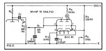
but the diode is reversed.  $R_1$  will now feed to pin 3 and pins 1 and 2 will connect to  $R_3$ .  $R_6$  has to be adjusted for zero, which will be *maximum* current through the meter, maximum signal will reduce the current to zero. Hence the meter can never be overloaded.
