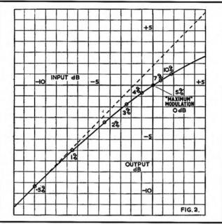
Fig. 2. Input/Output curve for tape, shown by full line. Dashed line shows perfectly linear characteristic. Percentage figures against circles show 3rd harmonic distortion at those points. The majority of properly recorded material lies below the 1 per cent. point on the curve.
