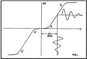
this method of recording the linear portion of the working characteristic is much longer, and the exact value of D.C. bias is less critical. It also has the advantage that the tape is automatically erased by the application of the saturating magnet, but the D.C. bias must always oppose the erasing field, so that polarity of erase magnet and head became important.
