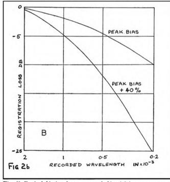
Fig. 2b Typical biasing losses, at peak bias (giving max. output at long wavelengths) and at peak bias + 40% (giving approx. 1-1 $\frac{1}{2}$ dB output loss at long wavelengths). 1 Thou' wavelength corresponds to  $7\frac{1}{2}$  Kc/s at  $7\frac{1}{2}$  i/s,  $3\frac{3}{4}$  Kc/s at  $3\frac{3}{4}$  i/s, etc. Bias set at 10 thou' wavelength.
