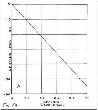
Fig. 2a Spacing losses, applicable to recording and playback in terms of wavelengths of separation.
