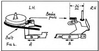
flywheel and RH turntable when the machine is "off", should press against the turntable with 75—100 grammes pressure when forward wind is engaged. The rewind pulley is also spaced at ½ mm from the flywheel, driving the LH turntable via a belt (see fig. 4). The pulley is held on a bracket, under spring tension of 20-25 grammes in the off position.
