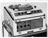
seen as well as heard! The latest stereo recorder from Vortexion is the CBL, with mixing of inputs, stacked heads and over 6 watts total output. Meter monitoring of bias and signal, and facilities for recording from track to track with additional signals, are features of note. Entirely separate low impedance micro-
