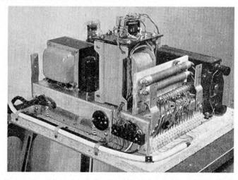
10 watt amplifier showing special output transformer on which is mounted the changeover relay. On the right is the tapped resistance for the projector motor circuit.
