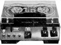
cells being loaded in interchangeable cassettes. Expected battery life is 30 hours for the motor (at 3\frac{1}{4} i/s) and 60 for the circuit. A line output provides a signal of one volt maximum, while a built-in speaker may be driven at 180 mW. Fast forward and rewind, a VU meter and response flat to 12 Kc/s at 7½ i/s make this a versatile high quality recorder. Price is 66 guineas.
