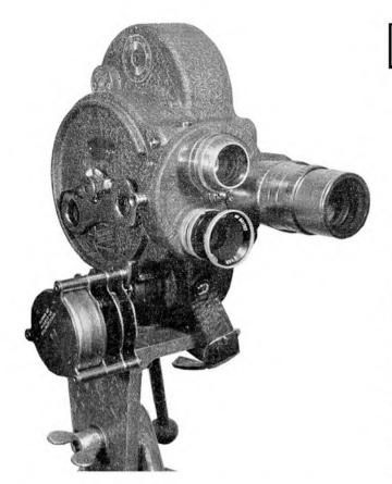
The above photograph shows a Bell and Howell 16 mm camera model 70DL fitted with a small generator for supplying the synchronising pulses.
