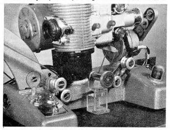
The projector showing film laced through recorder starting contact assembly (made of perspex).
