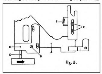
This dual relay arrangement gives a much more positive action, enables the use of simple relays, and allows a switch sequence ending in an "open" position.
