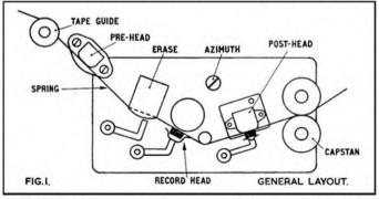
until the head is scanning the top tape track. Two 8 B.A. bolts, with a compression spring hold the head to the deck, and agile fingers the nut to the bit of bolt that penetrates the dark interior of the recorder. One head is fixed.
