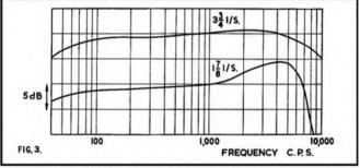
The slight lift at 4-5 Kc/s at the lower speed helps to compensate for the sharper high note cut off. Peak level recording tests showed that a level 11 dB above test tape level was recorded when the magic eye beams just touched, and that a further 2 dB increase in level could be recorded before the onset of waveform distortion.
