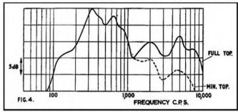
extent for a speaker or cabinet resonance in the low frequency range. In this case the microphone response does not help as the speaker peak is within the level range of the microphone.
