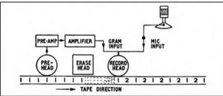
Fig. 5. Schematic diagram showing the super-superimposition process.
