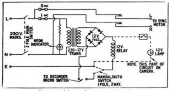
Diagram of the synchronous starting unit.
