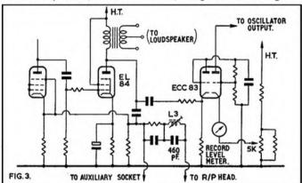
this preset and checking with a valve-voltmeter at the monitoring socket, when these recordings are played back it will be heard that the output signal rises as bias is increased. The correct setting is slightly higher than that producing maximum signal output
