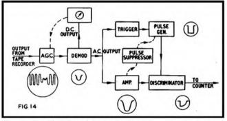
Fig. 14: Simplified block diagram of typical dropout counter circuitry, explained at length in text. Circular insets indicate typical waveforms expected at these points.
