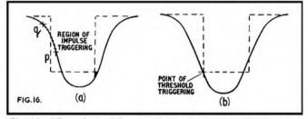
Fig. 16: Effect of two different methods of triggering reference pulse: (a) Impulse Triggering. (b) Threshold Triggering. Apparent differences in fluctuation length require shorter reference pulse length in (b) to produce same counting condition as in (a).
