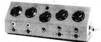
inputs are high impedance, and the output impedance is 600 ohms, up to 200 mV, suitable for gram input of a tape recorder. The model has two high-level and two low-level inputs and built-in power supply. The mixer is manufactured and distributed by Esisolder Iron Company Ltd., 98 Dominion Road, Worthing, Sussex.
