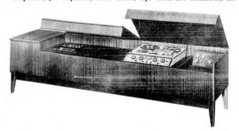
Lowline Five has pneumatic lid stays and adjustable mounting boards. The cabinet is finished in satin mahogany. The amplifier is housed in a separate, ventilated compartment to prevent hum and overheating. Overall size is  $81\frac{1}{2}$  in. long x 22 in. wide x 16 in. high. Price: £34 13s.
