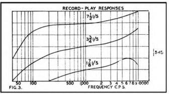
tion: at the two lower settings the high frequency response was cut by approximately 10 and 20 dB at 10 Kc/s. The 700 c/s peak is a cabinet resonance, and the 250 c/s peaks are speaker cone resonances which have been pushed up in frequency due to the added stiffness of the air in the compact cabinet.
