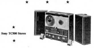
T ELLUX (Hi-Fidelity Division) recently announced a new Sony tape recorder, the *TC500*. A four-track, stereo machine it has speeds of 33 and 71 its, and incorporates sound-on-sound, automatic stop, and an automatic tape-lifting device. Independant recording and playback amplifiers provide a response of 30 c/s to 18 Kc/s at 71 i/s. A belt-less drive mechanism enables it to be used horizontally or vertically.
