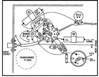
Fig. 2. Layout for EF86 input stage using anti-microphonic holder (with normal holder the screws come opposite sp and h pins, in which case use sp for earthing instead of s). See fig. 3 for circuit.
