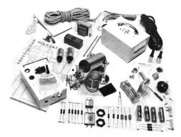
1. Here is the complete kit of parts, as unpacked. In the centre of the picture are the main components of the microphone. All the larger items make up the power pack. The locations of most of them can be seen in the other photos.
