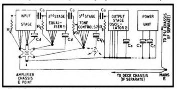
**Fig. 4.** Principles of earth wiring of amplifier in simplest form; see text for details. Cs - smoothing capacitor, <math>Cd = decoupling, Cr = reservoir.
