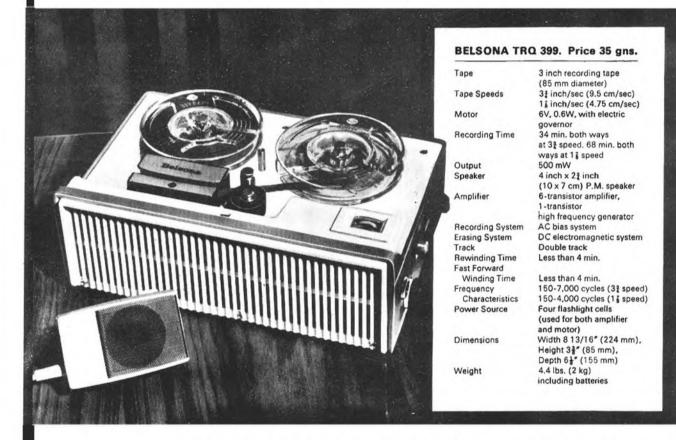
Compact Belsona portables offer the enthusiast many features previously found only in standard models. 'Hitachi Ring Base Transistors' ensure full tone and volume. Level Meter guides correct recording and shows how much battery life remains. The sensitive Dynamic Microphone can be operated by remote control. And there's no warm-up needed, transistors permit immediate recording and play-back.
