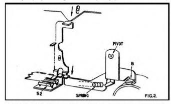
on a lever. which slides as the speed-selector knob is turned. The idler wheel is mounted in a bush which is raised and lowered by the ramp, to contact the appropriate step on the motor pulley.
