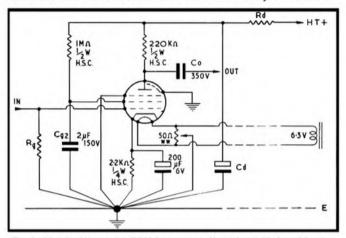
Fig. 3. Circuit of low-noise EF86 input stage. Note that grids 2 and 3 are returned to earth, not to cathode. Co and Cg2 must be paper or good metallised paper, metal cased. The 50 ohm WW pot is adjusted for minimum hum under working conditions. Values of Co, Cd and Rd depend on overall circuit arrangements.
