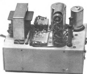
6. The finished power unit. Comparison of this photo with picture 3 shows the result of adding the prepared items of photo 2. There is very little under-chassis wiring. A straightforward job.
