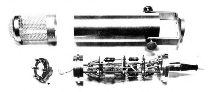
7. Sleeving is recommended, but our constructor preferred bare wires for simplicity, except at the 5-pin plug and where there is danger of contact with chassis via metal valve base ring. Gentle tension holds bare wires rigid. Terminal wires of resistors are used as wiring. The assembly is now slid into the case. Top plate (by solder tag) is screwed down on the rods. Tag is screwed to capsule, which is locked by grub screw, and gauze cap fitted.
