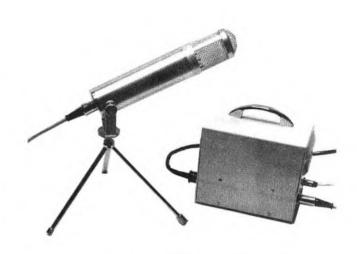
4. Here is the finished job. It looks good and it is good. The construction of the microphone/pre-amplifier unit demands really clean, careful work. The foil diaphragm is now supplied in finished, capsule form, thus obviating the most delicate work. Total time taken was 10 hours.
