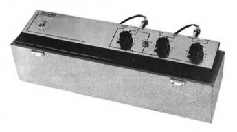
The level of echo is varied by a control which alters the ratio between reverberant and direct sound. The input signal is split along two paths, one of which receives delaying treatment before merging once more with the unaltered signal.
