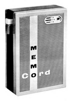
the red button continuously while recording, and when the button was released, both motor and amplifier circuits were disconnected. This was a simple safety measure which was superseded by a more practical record lock on later machines. Depressing the white or cream button for replay was a normal hold action which is neutralised by a touch on the red button.
