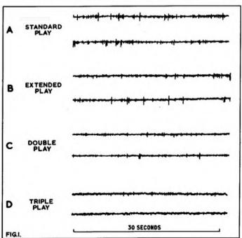
fairly frequent but this behaviour is typical of Standard Play tape, where the relatively thick base lifts the whole tape away from the head if a minute surface imperfection or dust particle comes between the head and the tape.
