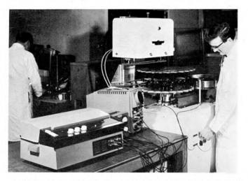
An MR800 Labcorder being used to record the vibrations of bearings and mountings of a Wehmiller Bottle Inspecting Machine.
