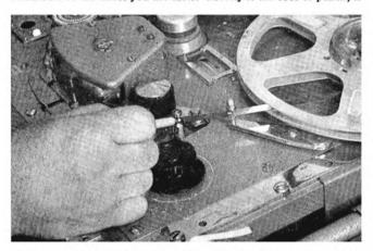
Above: If the playback head is inaccessible, the chinagraph mark can be made alongside a convenient guide; the distance from head to guide enables calculation of the cutting position. Photo on page 397: Daphne Oram, composer of musique concréte, makes full use of splicing techniques to produce the unearthly from everyday sounds. Both illustrations by courtesy of the BBC.
