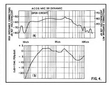
The Mic 60 (stick) and Mic 55 (lapel) cases can each be fitted with crystal, ceramic or magnetic inserts so that figs. 1, 2 and 3 cover the whole family of units using these inserts. The Mic 39 Dynamic uses a West German insert and is only available in a black stick case.
