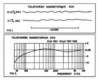
this little machine beginning to 'show through', and will be wondering if further tests uncovered any outstanding fault which modified my initial impression. I can assure them straight away that my measurements only served to confirm my opinion. Seldom have I tested a recorder where things were so 'right'.
