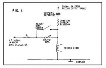
energised from the anode circuit of the record output valve through a coupling capacitor and highish value resistor, whose job it is to keep the record current in the head at a fairly constant level at all frequencies. The HF bias signal is fed into the head usually through a resistor (fixed or pre-set) given as R1 in the circuit. Now, the idea is to break this feed and insert a variable resistor and simple parallel switch.
