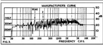
Fig. 3. Combined direct and reverb. response curves
