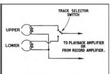
Fig. 6. Typical \fraction track head switching arrangement.
