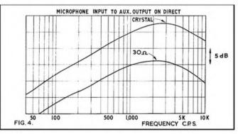
was short circuited by the test set up. Signal/noise ratios on either microphone input were only 30dB due to the high transistor noise.
