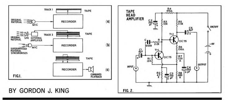
LAST month's article finished with a discussion on how one section of a  $\frac{1}{4}$ -track head can be arranged to monitor a recording previously made on one track while the other section of the head is actually producing a recording on another track. We saw that this technique makes it possible to synchronise the material on two tracks so that on replay the simultaneous outputs from the two head sections can be mixed (i.e., connected in parallel) at the input of the playback amplifier.
