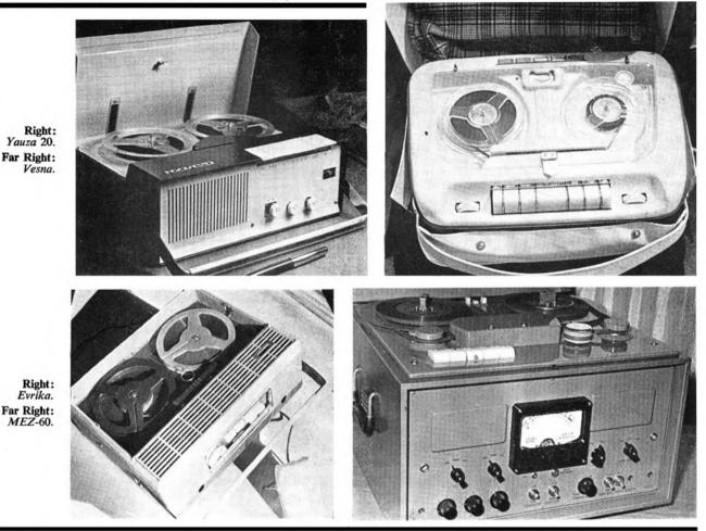
phone, radio receiver and gramophone. One motor is used for track switching. Double-purpose amplifiers and dual-purpose heads are used for recording and playback. The recorders can be powered from an AC mains supply and have two loudspeakers.
