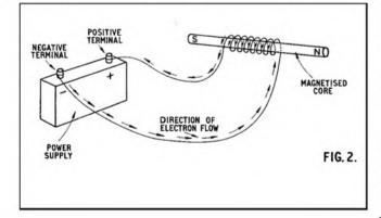
reverses the polarity of the magnetic field, an iron core now having a North pole where the South pole was situated, and vice versa. Were the battery in **fig. 2** to be replaced with a power supply continuously alternating from positive to negative and back to positive (AC), the polarity at each end of the core would change in sympathy.
