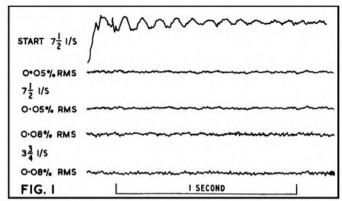
The rubber disc which couples the motor shaft to the flywheel is rather soft and there is a damped oscillation at about 10 c/s which persists for about one second when the motor is switched on, see top trace fig. 1. This mass-compliance resonance can be shock-excited by touching the tape as it leaves the supply reel or by bad spooling which may cause the tape to touch the reel flanges occasionally.
