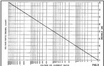
DEFINING the Decibel without recourse to mathematics is not the easiest of tasks. To begin with, the Decibel is not a unit in sense that Volts, Amps or Watts are, but a means of measuring ratios.
