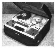
ing controlled independently on each channel. Each machine is supplied with a frequency response curve sheet produced on *Brüel & Kjaer* test equipment. Claimed frequency range is 20 c/s-20 Kc/s at  $7\frac{1}{2}$  i/s, with wow and flutter of  $\pm 0.08\%$  RMS. At  $3\frac{3}{4}$  i/s figures of 20 c/s-15 Kc/s with  $\pm 0.15\%$  RMS are specified. An original feature of the 22,
