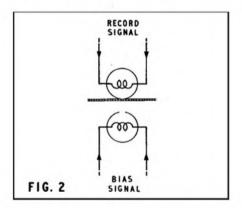
The frequency of the bias should be at least four times the top frequency handled by the machine. As the bias is derived from the same oscillator as that providing the erase signal, its frequency ranges from about 35 Kc/s to about 80 Kc/s, or higher than this in some professional models. One of the problems of direct bias lies in impairing the top frequency response (see under CROSS-FIELD RECORDING).
