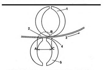
This is the Crossfield Head—only Akai has it. 1 signal head. 2 bias field. 3 direction of tape travel. 4 signal field. 5 bias head. 6 bias head retracts automatically on playback.
