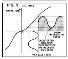
it passes the recording head gap, its response becomes very complicated. As it recedes from the point of maximum field intensity within the gap, it is in effect subjected to a decreasing alternating field, which introduces a certain amount of demagnetisation. The extent of this self-demagnetisation depends upon the number of signal cycles which occur while the tape is in the gap. So it will increase with frequency and decrease with increasing tape speed.
