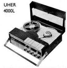
MANUFACTURER'S SPECIFICATION. Twintrack battery portable recorder. Tape Speeds: 71, 31 1% i/s and 1% i/s. Frequency Range (respective): 40 c/s - 20 Kc/s, 40 c/s - 17 Kc/s, 40 c/s - 10 Kc/s, 40 c/s - 4.5 Kc/s. Signal-to-Noise Ratio: 55dB. Wow and Flutter: ±0.15% at 7½ i/s. Output Power: 1W. Power Supplies: Five torch cells or Z211 rechargable battery. Z114 power unit/battery charger available. Price: £108. Distributor: Bosch Ltd., 205 Great Portland Street, London, W.1.
