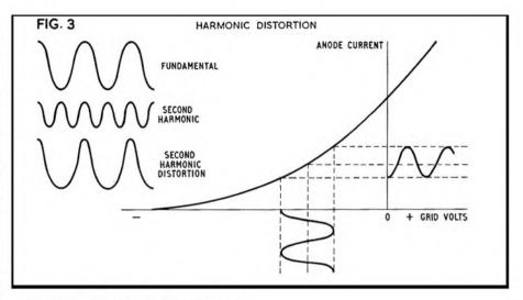
Harmonic and amplitude distortion are two more forms of distortion which are produced by curvature of the amplifier characteristic. Even the 'straight' portions of most amplifier characteristics have a certain amount of curvature. The pentode valve is a particularly bad offender in this respect.
