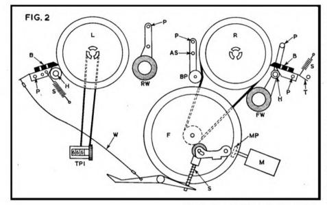
Simplified layout of drive and braking system-Points discussed in text are pivot P, spring S, tongue T, forward wind idler FW, rewind idler RW, motor M, motor pulley MP, bearing pulley BP (engaging flat belt), adjusting screw AS, tape position indicator TPI, hold-off pin H, left brake wire W.
