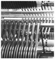
Part of the slitting mechanism, here showing cutting of 2in. computer tapes.
