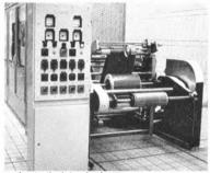
Leaving the drying chamber, the magnetic f.Im is wound into blocks.
