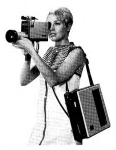
SONY BATTERY VTR ETAILS of the Sony battery video recorder have been trickling into the country during the last few months, followed, now, by the first illustrations. The equipment produces tapes for reproduction on the £350 Sony mains recorder and does not itself have replay facilities. Of particular interest are the miniature CRT view-finder and microphone mounting arrangement; price in the USA is some £430.
