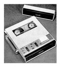
View of the TP1002 showing second speaker detached. This fastens to the recorder to provide forward and rear-facing units.
