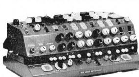
Fig. 3—The top section hinges to give access to the circuits.
