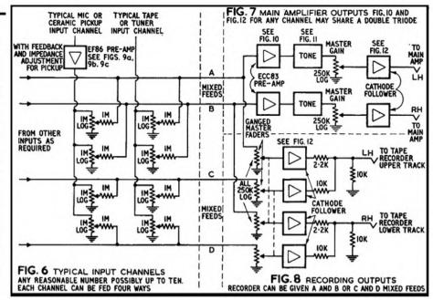
the arrangement and readers are referred to Graham Balmain's article on 'Hum and Noise in Tape Recorders' in *Tape Recorder* (December 1963). Layout is important to avoid lowering the possible standards and fig. 9b shows the arrangement suggested by Mr. Balmain. F1 should be of a value suitable for the secondary impedance of the microphone transformer being used. High stability resistors are always worthwhile.
