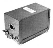
pulse generated within the camera to an inaudible pilot signal. This signal is recorded with the film sound on to a conventional single-channel tape recorder. The R.1 is battery powered, measures  $10 \times 5 \times 4$  cm, and incorporates a miniature jack pulse input and three-pin DIN tape output. A battery life meter is also fitted.
