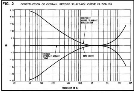
A S lower tape speeds become more common for sound reproduction from magnetic tape, the difficulties in maintaining a satisfactory dynamic range are accentuated. The limitations are imposed partly by the increased relative noise level associated with a reduction of the tape speed, and partly by the increased pre-emphasis required for obtaining a given frequency range at a satisfactory signal-tonoise ratio.
