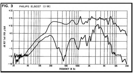
show the free field sensitivities of both these microphones. They are substantially similar, the differences in the back response of the two microphones being due to normal manufacturing tolerances. The response is flat from 200 Hz to 10 kHz, and the usable response is from 100 Hz to 20 kHz.
