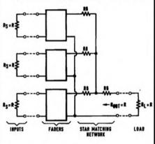
FIG. 13 EQUIVALENT CIRCUITS FOR CALCULATION OF THE MATCHING LOSS
