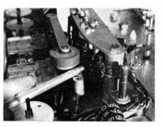
If neglect is the basic cause of trouble, the solenoids may be sluggish, and more than once this has led to replacement when all that was needed was cleaning and thorough lubrication. The slug must slide freely, and can be removed, cleaned with spirit, with the barrel similarly treated, and then reassembled with a smear of Molyslip. As with all lubrication, a little in the right place is the secret, not liberal application.
