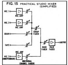
to allow each source to be controlled by any group fader.
