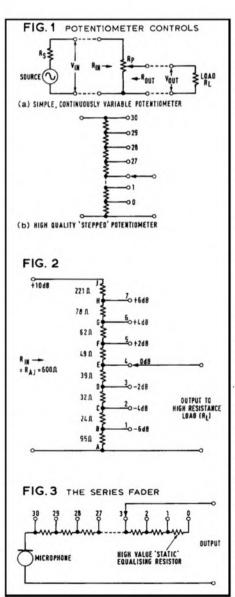
differences, and 0 dB is any arbitrary value.) This potentiometer is designed to have an input resistance ( $R_{\rm in}$ ) of 600 ohms, and the load resistance ( $R_{\rm L}$ ) is assumed to be high compared with  $R_{\rm P}$  so that the shunting effect of the load on the potentiometer is negligible.
