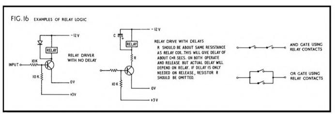
inserted. Some form of indicator will also be needed in order to determine the logic levels in the various parts of the circuit. The best way of doing this is with a 12 V meter (which may be a 1 mA meter with a 15 K resistor in series), since this will show small discrepancies in the voltage levels. Failing this, the circuit show in fig. 17 may be used. It will anyway be very useful if four of these circuits could be made in order to show the state of the counter.
