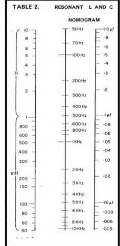
PLACE A STRAIGHT EDGE BETWEEN SELECTED VALUES IN ANY TWO COLUMNS AND READ OFF THE THIRD, UNKNOWN PARAMETER IN THE REMAINING COLUMN. FOR COIL WINDING DETAILS SEE TEXT L.H. COLUMN
