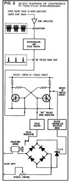
shorter time after the on pulses, and automatically correct the speed of the motor. In this manner the motor is electronically locked to the pulses on the tape by what is known as the mark space ratio of the pulses and, therefore, the projector remains in precise sync to the
