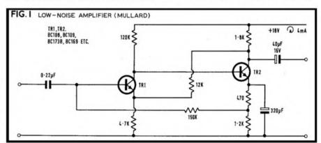
the output from unit A should be 1.5 to 3 times
