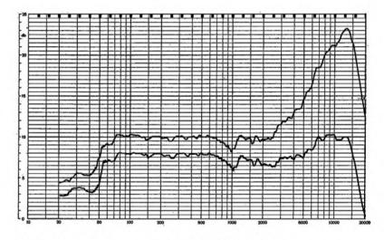
B & K frequency response traces with 0.25  $\mu$ F capacitor at output (lower curve) and without capacitor.
