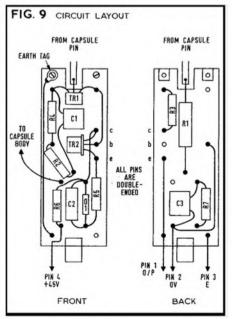
the body as possible. After soldering the FET into the circuit, the wire is removed. For similar reasons, do not touch the capsule centre pin while installing it, and tighten the grub screw with a screwdriver the shank of which is temporarily connected by a loose lead to the O V line (Pin 2 of the connector).
