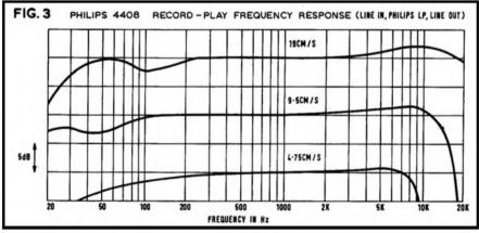
This should be borne in mind when playing prerecorded tapes at 9.5 cm/s into wide-range external amplifiers and speakers. A slight touch of top lift will be required at this speed. If the tapes are played on the machine's own speakers, the treble tone control can be left near the mid setting.
