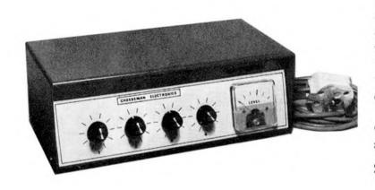
\*Mains powered \*Two input levels per channel; low level for microphone, high for gram or tape \*High and Low level outputs \*Separate pre-amps for each channel for low noise \*7 Mullard silicon transistors \*Accurate Level Meter for operation remote from recorder
