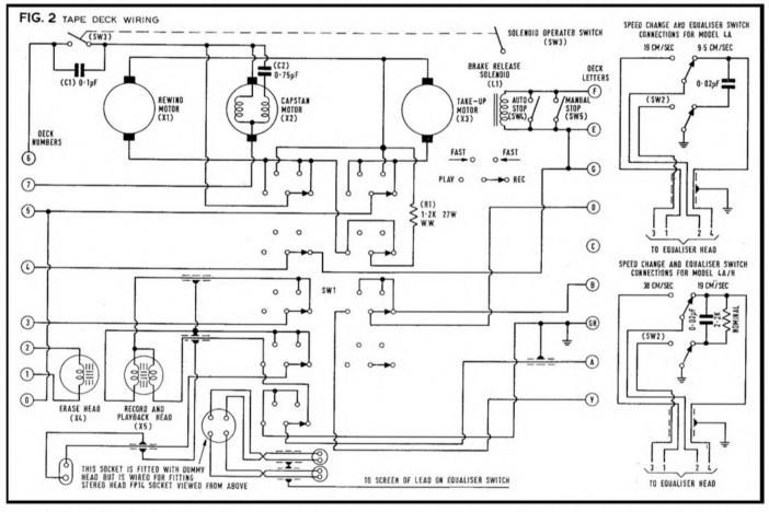
gested in the original Wright & Weaire blueprints. Careful comparison with later Ferrograph models reveals that there are several minor alterations, such as the detail of the meter circuit and the equaliser network between first and second stages. Fig. 2 goes on to show the deck wiring, including the switching which has given some people an awful lot of bother when they have had to rewire a broken switch.
