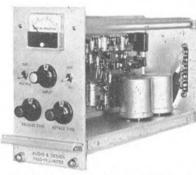
A Mk. 2 version of the well established F600 unit. Gain within the system is normally 25dB with output level of 0dBm (+8dBm to order). Compression ratio better than 25:1; variable attack and release controls with auto network. Noise -70dBm. Response: 10Hz-50kHz for -3dB. Distortion: 0.1% for 25dB reduction at IkHz.
