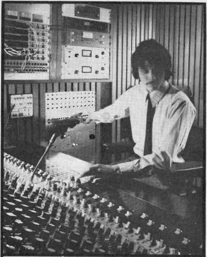
Robin Cable at one of the Sound Techniques' mixing desks used at Trident Studios, now equipped with twenty-two A301 units on two sixteen track machines.
