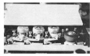
Fig. 4 Head gate and pressure pad arrangements. Note guide positions.
