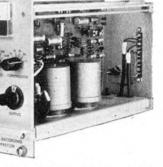
The new F700 Compressor provides a range of compression slopes from less than 2:1 to greater than 25:1; switched attack control for special effects; switched release control from 25mS. The threshold level is switched with compression slope to provide a constant level of output for 17dB reduction. Normal output level (unattenuated) +8dBm. Noise better than -75dB below Limit level Distortion: 0.1% for 25dB reduction.
