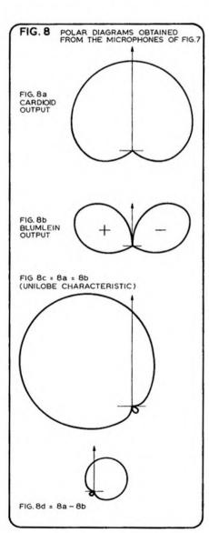
capsules placed next to one another can provide a coincident four-channel stereo output with excellent channel separation at mid-frequencies.
