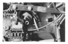
Fig. 7 Original cable-and-nipple drive was superseded by a sheathed cable but still gave trouble so . . .
