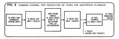
tracks set to match the playback levels on the auditorium stage. At the same time the four tracks containing the chorus were mixed together in pairs with the four tracks containing the ambience and third violins, resulting in a 12-track audio master leaving four tracks available for the pre-programmed lighting cues.
