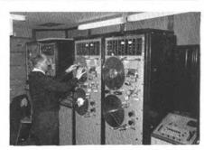
line, a Westrex compressor used to keep the dynamic range within reasonable limits, levels being controlled on a four-channel Vortexion mixer. The main recording was made on a Gaumont Kalee 16 mm edge track machine and backed at 19 cm/s on a TRD recorder. A further recording was made on a Grundig *Stenorette* for transcription purposes. In the speech cubicle are a telephone, a ribbon microphone for the 'rear' voice, and a GPO telephone matching unit.
