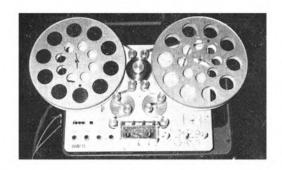
Sondor M3 sprocketed film sound recorder
