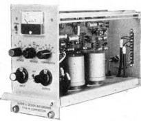
The new F700 Compressor provides a range of compression slopes from less than 2:I to greater than 25:I; switched attack control for special effects; switched release control from 25mS. The threshold level is switched with compression slope to provide a constant level of output for I7dB reduction. Normal output level (unattenuated) +8dBm. Noise better than -75dB below Limit level Distortion: 0.1% for 25dB reduction.
