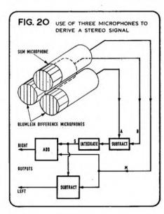
distance d is 2.5 cm, the three-microphone arrangement gives a reasonable unilobe characteristic and excellent stereo separation up to a frequency of  $\frac{1}{2}(c/d) = 6.8$  kHz, and the stereo separation virtually disappears at a frequency of about (c/d) = 13.6 kHz. Thus good stereo can be obtained by using the Blumlein difference technique with three microphones, even with a microphone separation of 2.5 cm. The results with smaller microphone separations will be even better.
