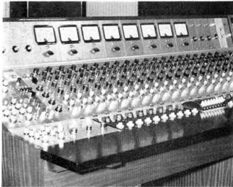
'RIDENT Studios in St Anne's Court, Soho, were designed by Sandy Brown, and are among the most modern and wellequipped studios I have visited. The main control desk was built by Sound Techniques to Trident's specifications and has 20 input channels and 16 outputs. In addition, there are four auxiliary outputs to which sources can be selected and echo effects added. These four outputs are normally used only for monitoring purposes.
