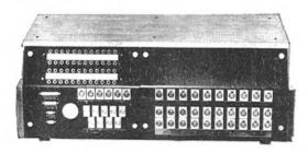
The Neve BCM 10/2 marks a new departure into the field of sophisticated audio control. It embodies ten full mixing input channels and two output groups and is conveniently transportable.
