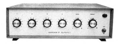
100 WATT ALL SILICON AMPLIFIER. A high quality amplifier with 8 ohms-15 ohms or 100 volt line output for A.C. mains. Protection is given for short and open circuit output over driving and over temperature. Input 0.4 V on 100K ohms.
