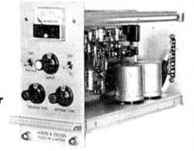
A Mk. 2 version of the well established F600 unit. Gain within the system is normally 25dB with output level of 0dBm (+8dBm to order). Compression ratio better than 25:1; variable attack and release controls with auto network. Noise-70dBm. Response: 10Hz-50kHz for -3dB. Distortion: 0.1% for 25dB reduction at 1kHz.
