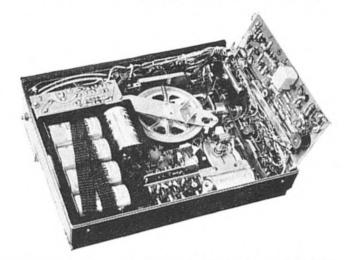
The usual trouble is contact points, and a clearance of 100 µm is required. Again, the only adjustment is the bending of the backing strips. I have never found this operation to be entirely satisfactory and avoid it wherever possible. We had a great deal of this to do on older Grundig recorders and used always to carry a stock of spare 'spring sets', finding this more economic than attempting to undo the 'bend and twist' efforts of our predecessors.
