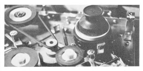
Above: One Sony version, where a combination of belt and pulley drive dictates clutch style. Basically a weight-dependent type but relying on the pulley drive for its efficiency.
