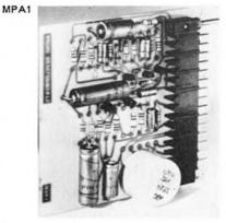
Both printed circuit cards will fit to a Painton 15 way connector. The connectors are fitted with polarising pins and they are connected so that either board can be inserted without any alteration to the common connections.
