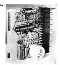
Both printed circuit cards will fit to a Painton 15 way connector. The connectors are fitted with polarising pins and they are connected so that either board can be inserted without any alteration to the common connections.
